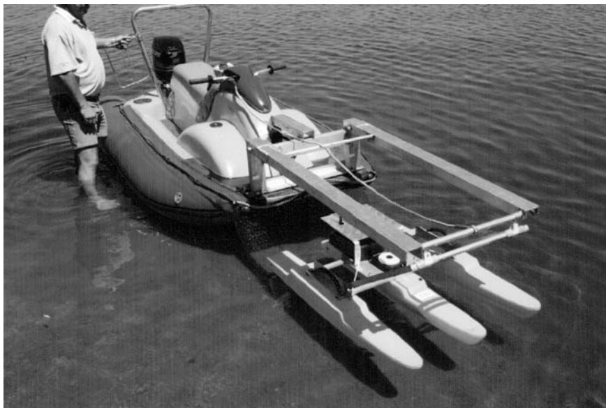
Figure 6.6(a) A small catamaran with aluminium jib-mounting for small boats. Source: Republic of South Africa.
