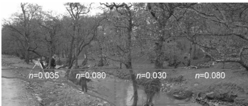
Figure 5.21 Estimating the Glen Ample flood in 2004, showing a diagrammatic view of the cross-section with the selection of three ' n ' values (Cargill, SEPA UK).
