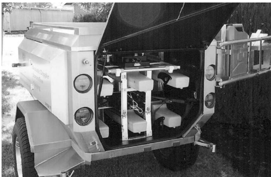
Figure 6.12 Customised off-road trailer accommodating the ADCP catamaran and equipment.
