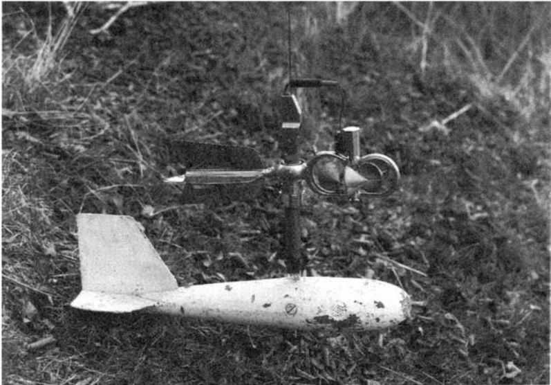
Figure 2.5 (a) Cup-type current meter (Price) and pigmy (mini) Price. (b) Watts cup-type current meter (shown with sounding weight and hanger bar for cable suspension).
