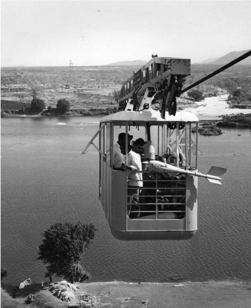
Figure 2.21 Electrically operated cable car with current meter and sounding weight.
