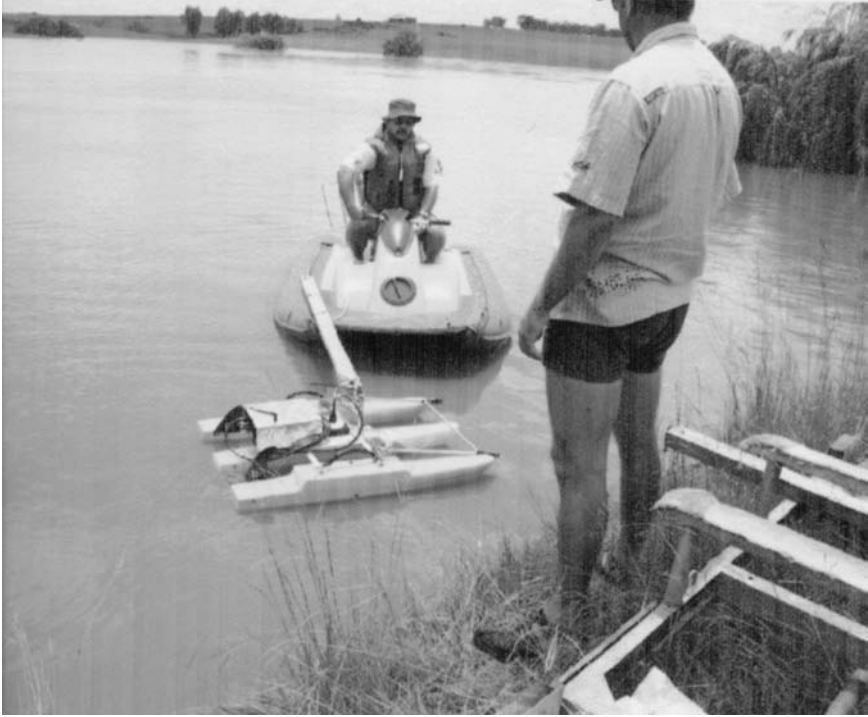
Figure 6.5(a) A small ADCP catamaran mounted on a small motor launch on the Vaal River at Gladdedrif.
