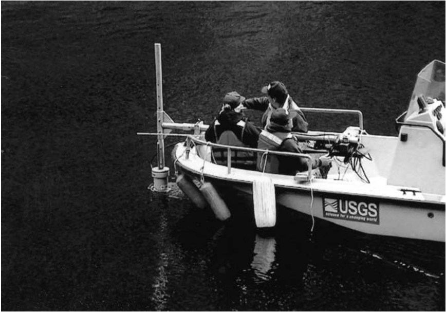
Figure 6.11(a) Gauging with a front (bow) mounted ADCP on a modern motor launch.
