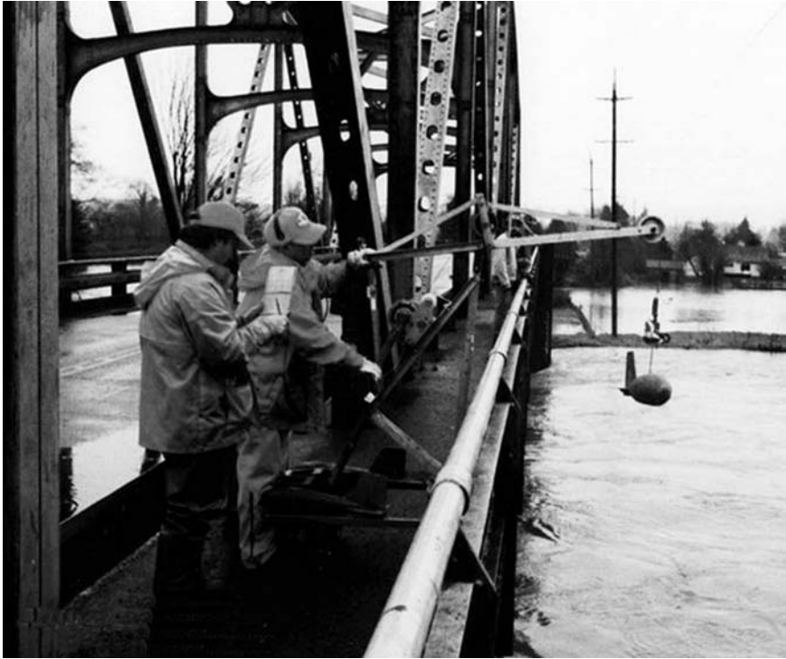
Figure 2.19 Single-drum winch on truck-mounted crane for gauging from bridge (Mississippi River).
