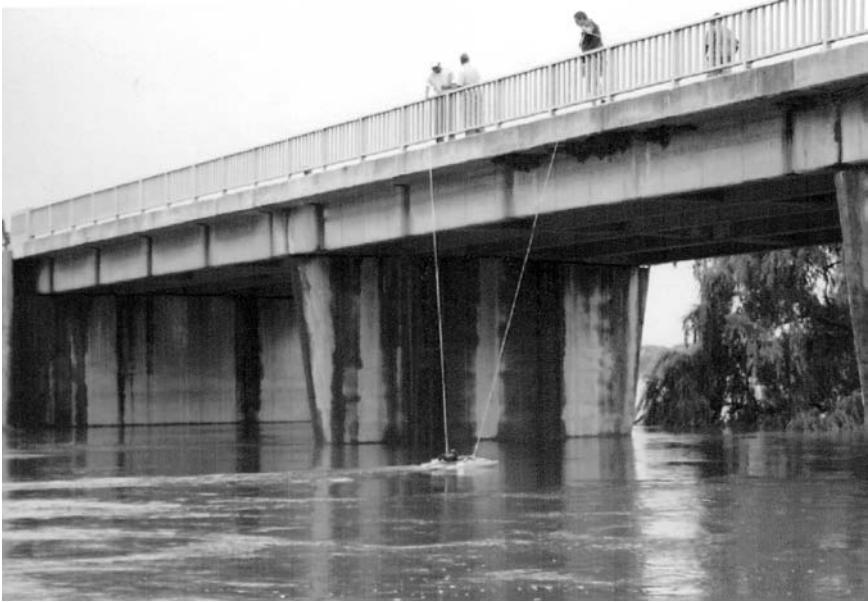
Figure 6.10 ADCP gauging downstream of bridge using small catamaran on the Vaal River at Blaukop.
