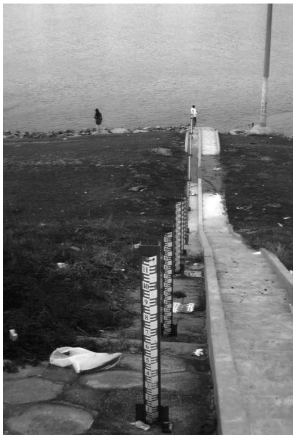
Figure 3.2 Vertical staff gauge installation with additional sections, Han River at Xian Tao, China.
