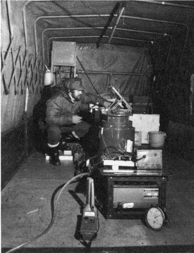
Figure 11.11 Complete injection equipment for a dilution gauging, housed in a truck.
