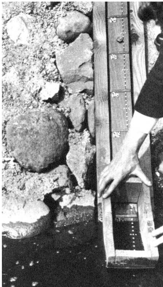
Figure 3.6 Portable stilling box to dampen wave action and facilitate reading of ramp gauge.
