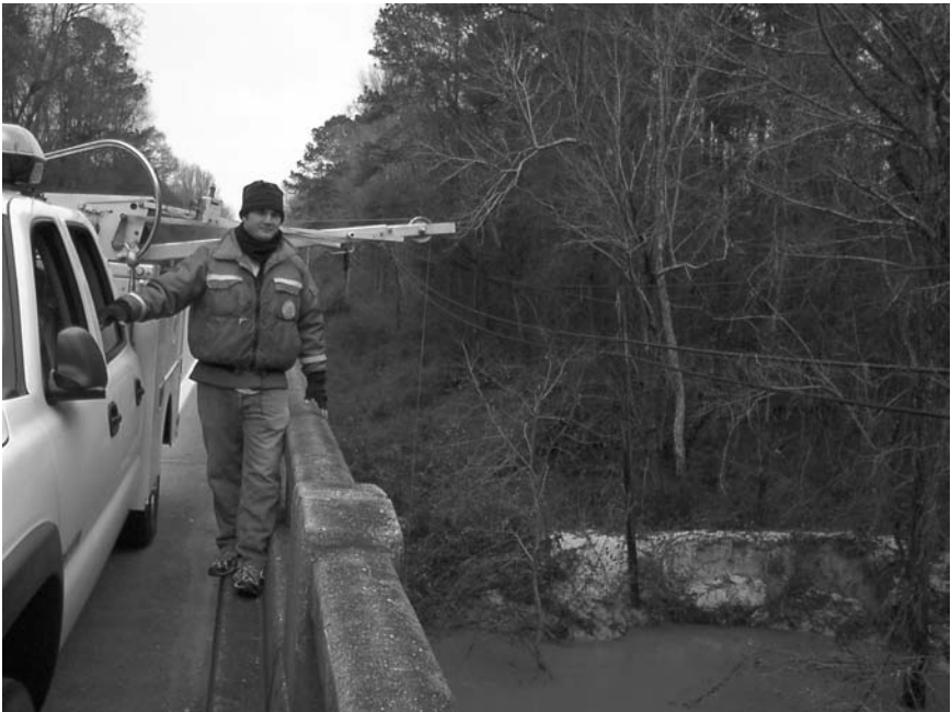
Figure 2.25 Bridge crane with four-wheel base showing boom in retracted position. Note protractor at outer end of boom to determine angle of suspension cable.
