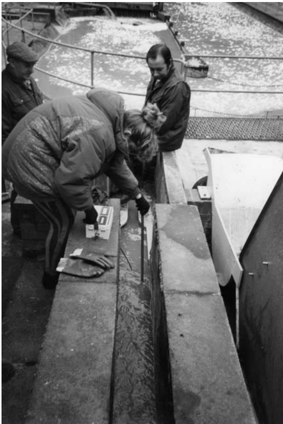
Figure 10.34 Small 100 mm rectangular standing wave flume under test.
