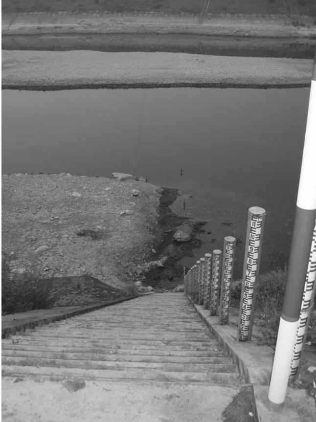
Figure 3.3 Staff gauges with additional sections for increased range of stage, Qing River at Gao Ba Zhon, China.
