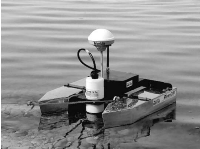
Figure 6.13 Details of a complete ADCP assembly of a SonTek catamaran with tow rope connection.
