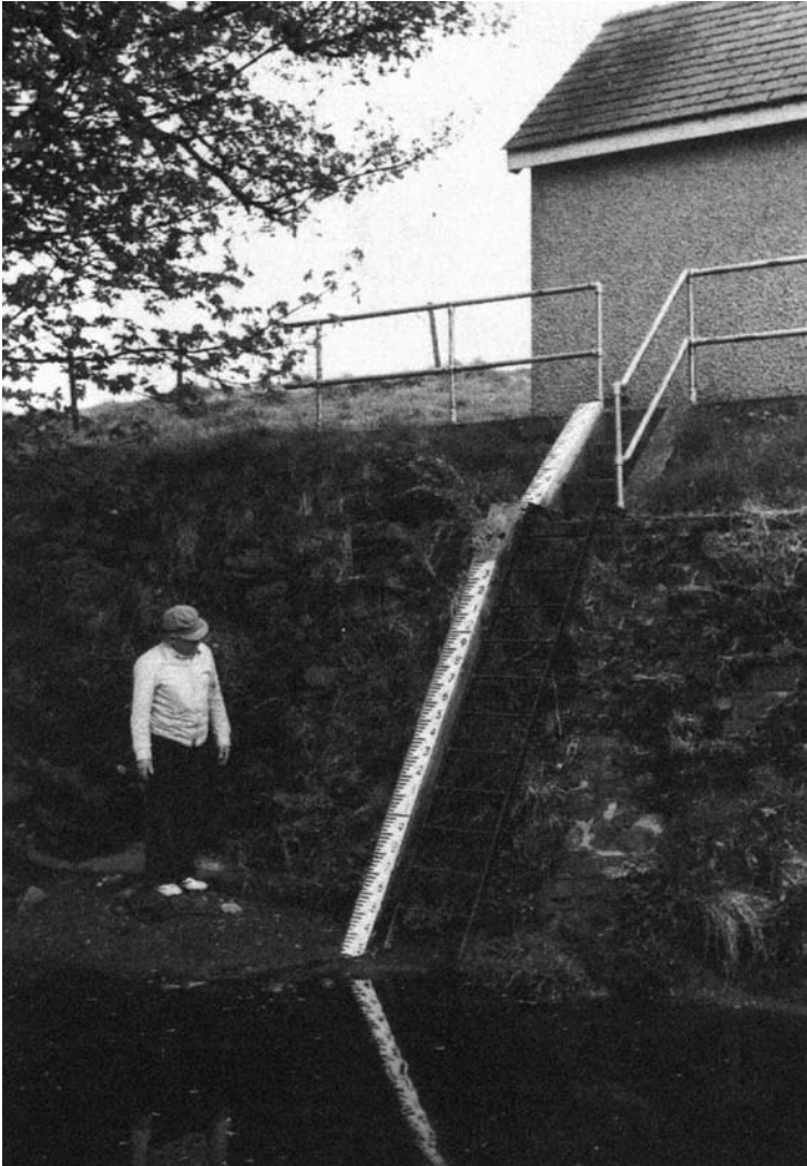
Figure 3.5 Typical ramp gauge installation.
