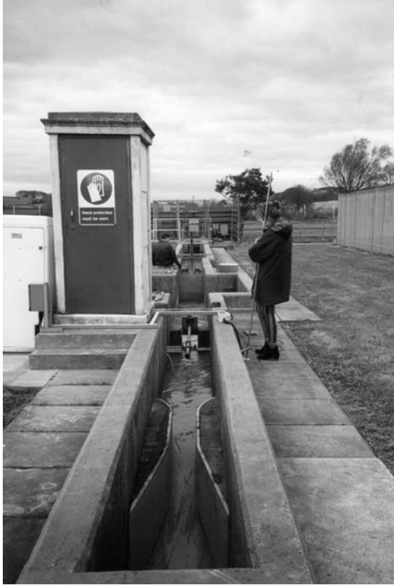
Figure 10.35 Small rectangular standing wave flume under calibration. Note electromagnetic current meter, 'Diptone' electric-tape gauge and 'look-down' ultrasonic water level gauge.
