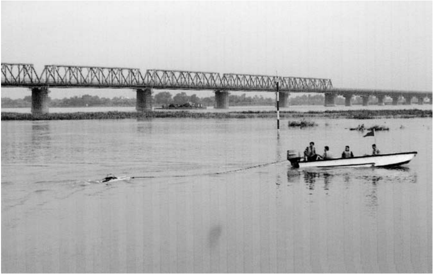
Figure 6.8 An ADCP gauging with motor launch and catamaran under tow cable on the Songhua Jiang River in China.
