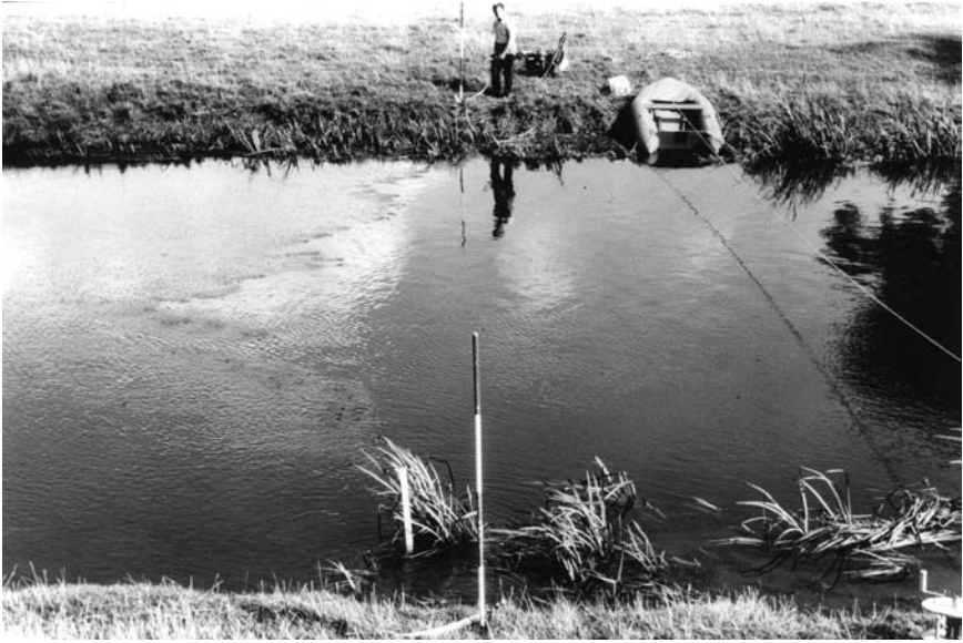
Figure 7.9 Typical gauging by rising bubble (air float) method: note the line of bubbles on the surface.
