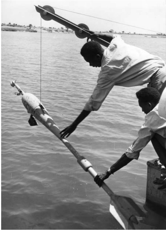
Figure 2.17 Current meter and sounding weight with current meter attached to nose of weight. Note ground contact device below weight.
