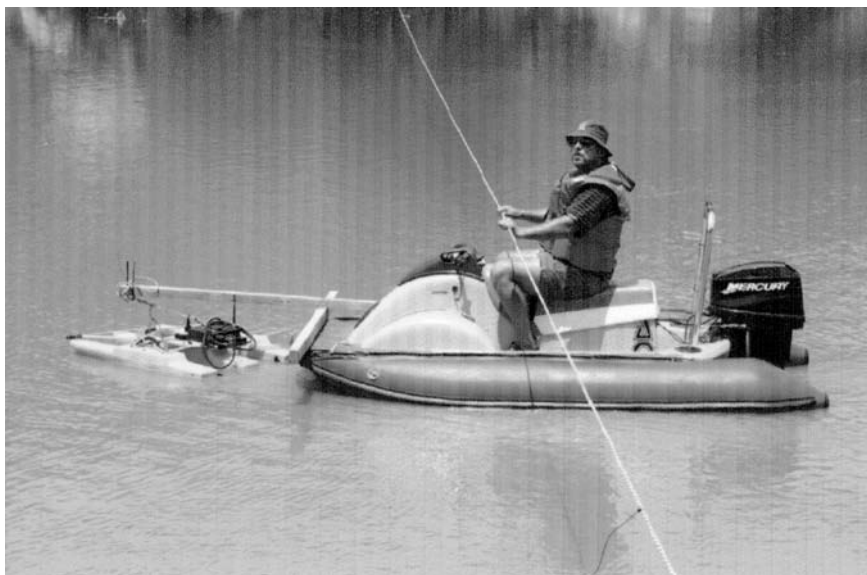
Figure 6.7(b) Details of the mounting of an ADCP with a motorised catamaran on the Vaal River at Goose Bay Canyon.
