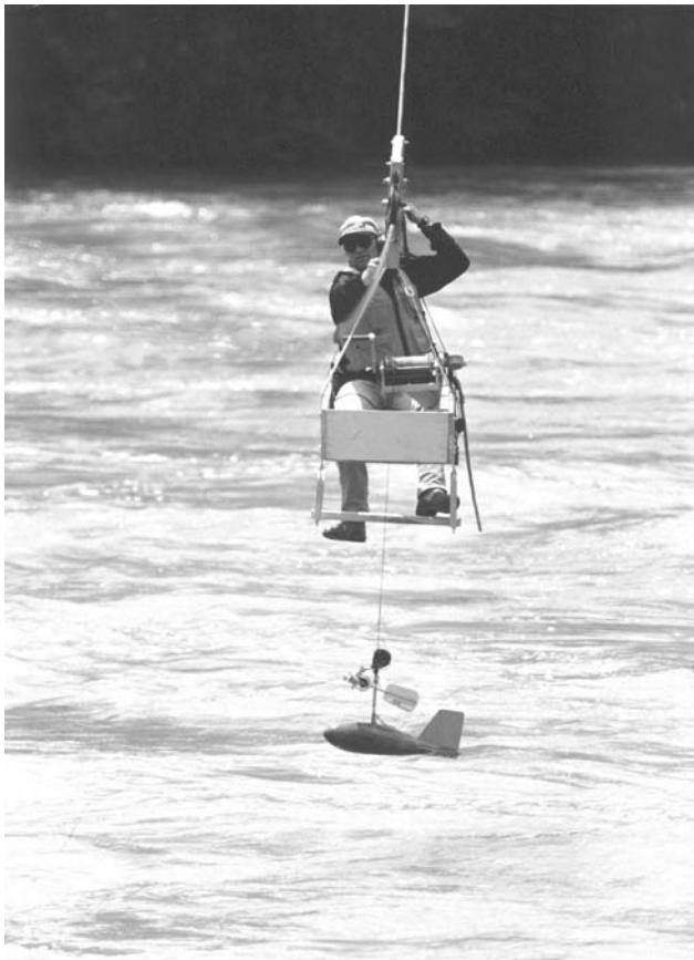
Figure 2.22 (b) Cable car operation on the Snake River at Idaho: cup-type current meter and Columbus sounding weight (USGS).
