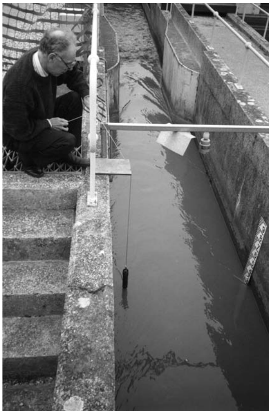
Figure 10.3 The photograph shows the electric-tape gauge (Fig. 3.8) being held against the datum plate to make a measurement of water level. As the buzzer sounds on contact being made with the water surface, the tape is read to the nearest millimetre. The distance from the datum plate to the bed of the channel being already measured by surveyors level, or other means, the depth of flow (head) is the difference between the two readings (no hump). The photograph also shows the staff gauge and an ultrasonic look-down water level gauge (see also Fig. 3.18) in the approach channel of a rectangular standing wave flume. Note the sun shade over the ultrasonic transducer to avoid faulty water level recording due to temperature change.
