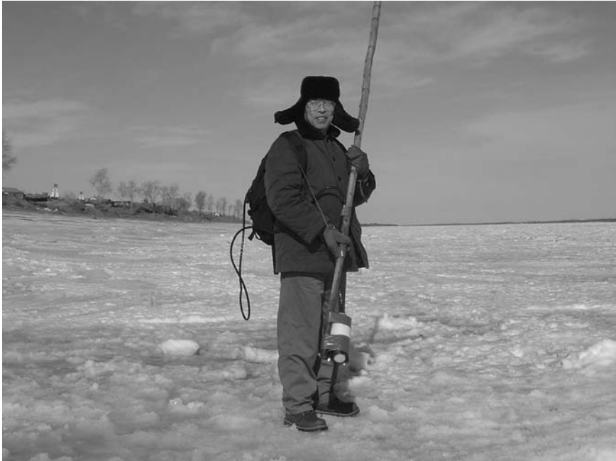
Figure 5.19 The SonTek ADCP River Surveyor 100 mm diameter transducer head being used as a hand-held current meter during a measurement under ice in the Amur River in China. Note software electronics being carried on site in operator's backpack.
