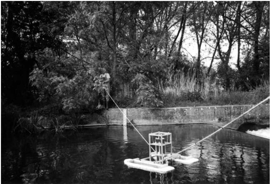
Figure 6.3(b) ADCP, in its simplest form for discharge measurement being moved across the river by an operator on each bank.
