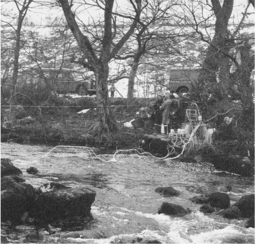
Figure 11.1 Constant rate injection dilution gauging by the multipoint injection method.
