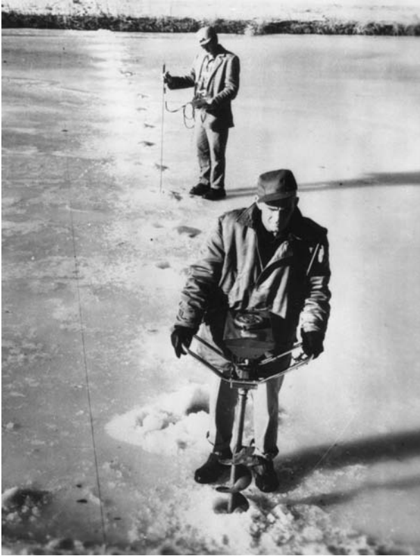
Figure 5.18 Drilling holes in ice (foreground); ice rod being used to support current meter for a velocity measurement under ice cover (background).
