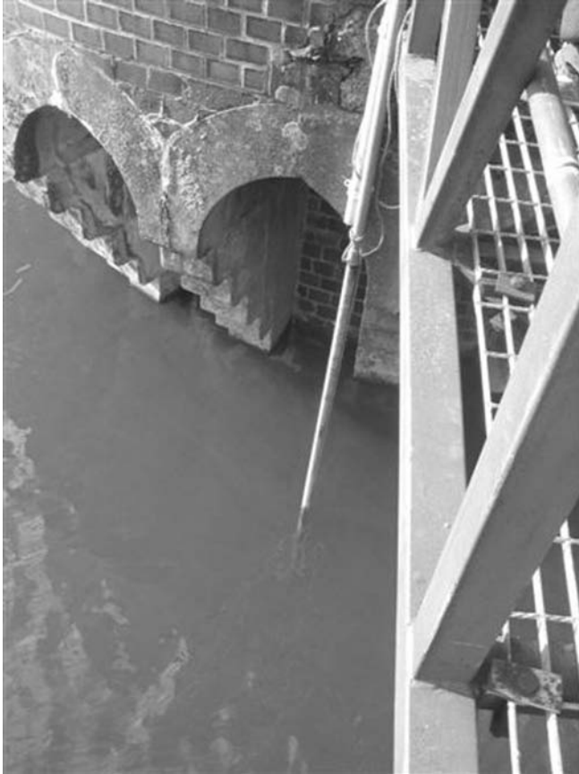
Figure 3.13 (e) Bubble gauge bubble pipe of bubbler installed at a dam.
