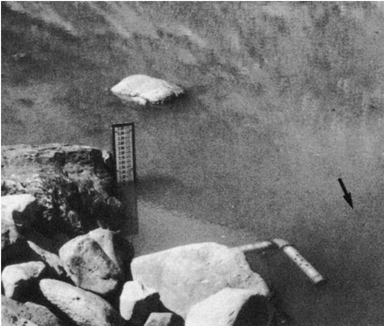
Figure 5.7 Typical installation of intake pipe fitted with static tube.
