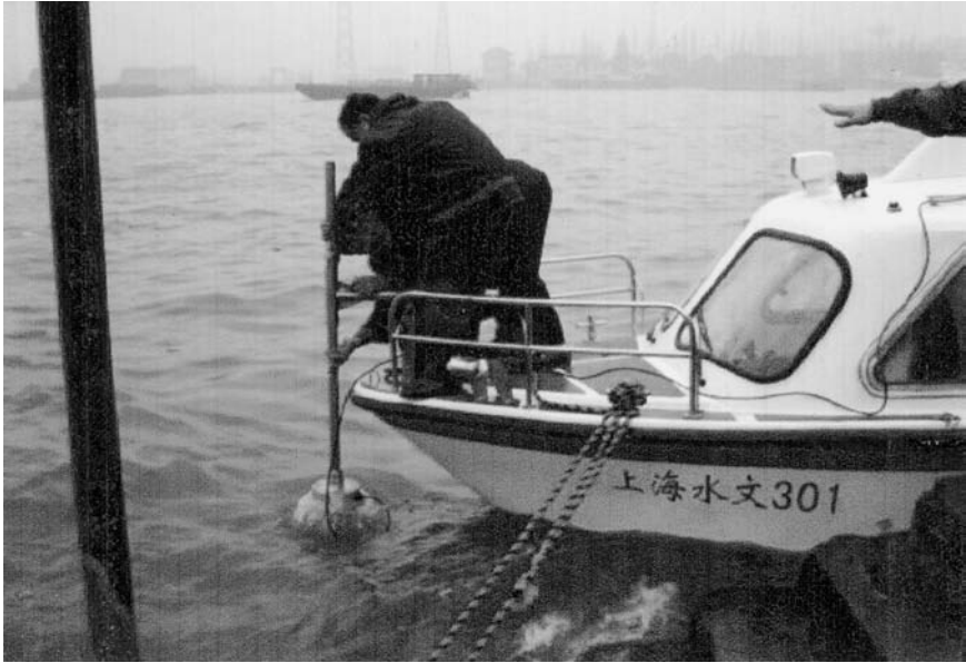
Figure 6.3(c) An ADCP mounted on a motor launch on the Huanpu River in China. Source: SonTek.
