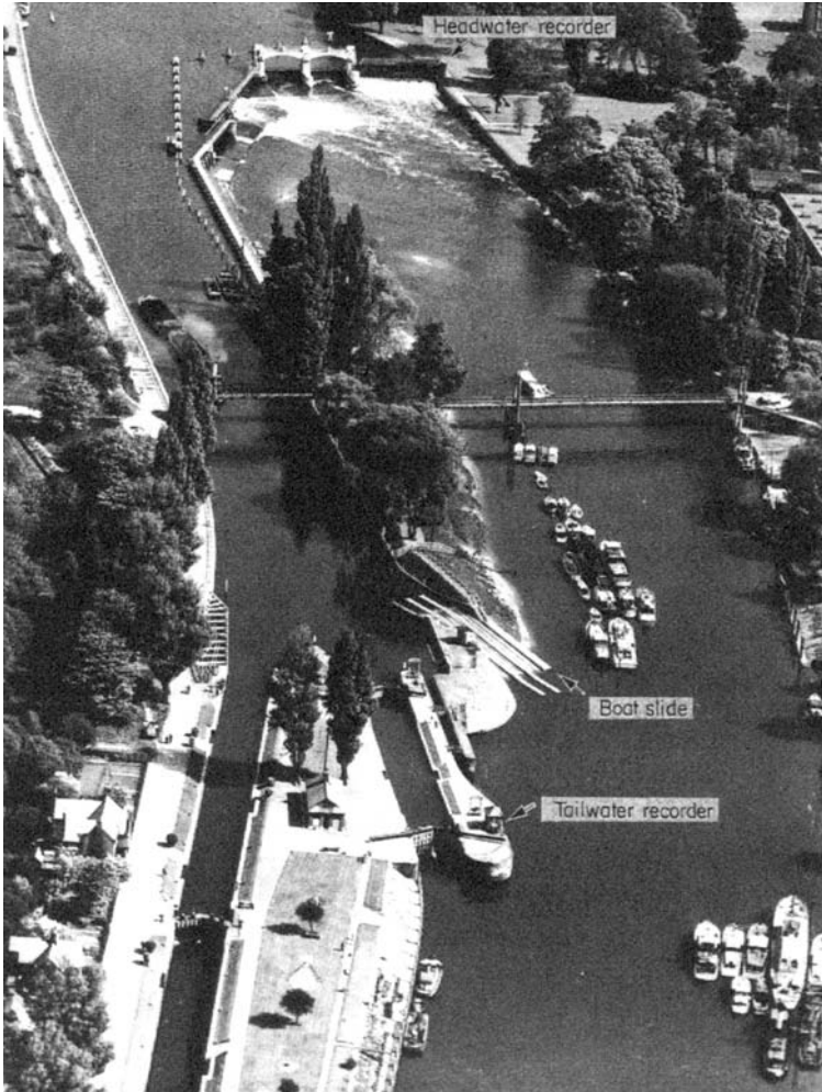
Figure 10.1 Aerial view of River Thames at London (Teddington Weir) used for streamflow measurement 1883–1982; weir comprises 34 radial gates, 37 sluice gates and a thin plate weir for measuring the lowest flows.
