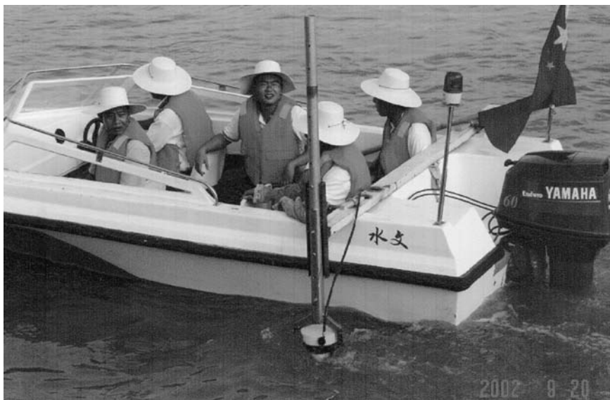
Figure 6.11(b) Gauging with a side-mounted ADCP on a modern motor launch on the Pearl River Estuary in China.
