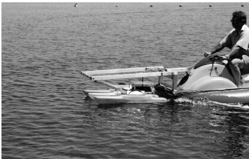
Figure 6.6(b) An ADCP gauging in operation. Source: Republic of South Africa.
